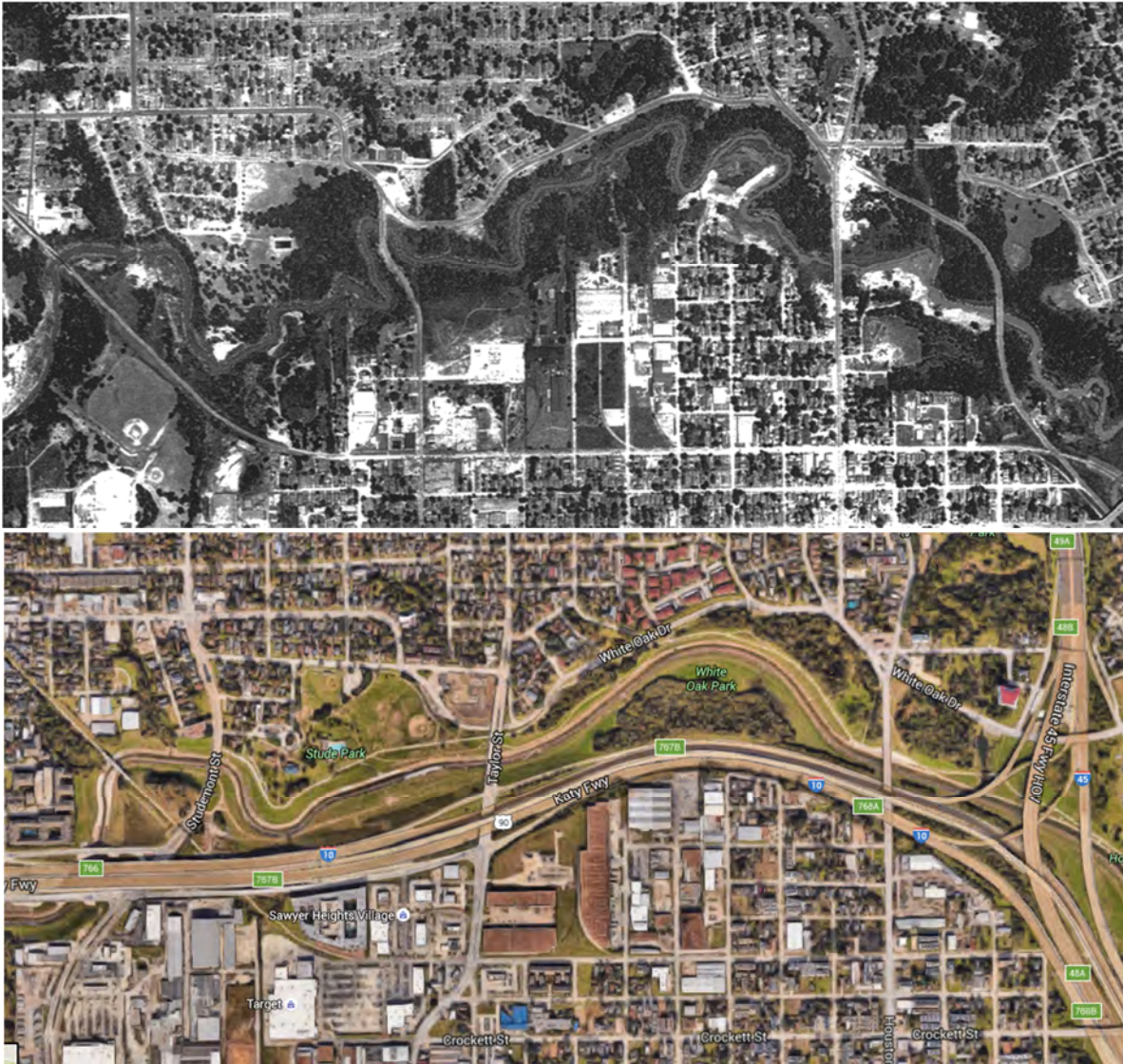
White Oak Bayou between Studemont Street and Houston Avenue, before and after channelization. The stream's course was straightened and most of the riparian vegetation corridor removed. Historic image courtesy of HCFCD, modern image courtesy of Google Earth.
